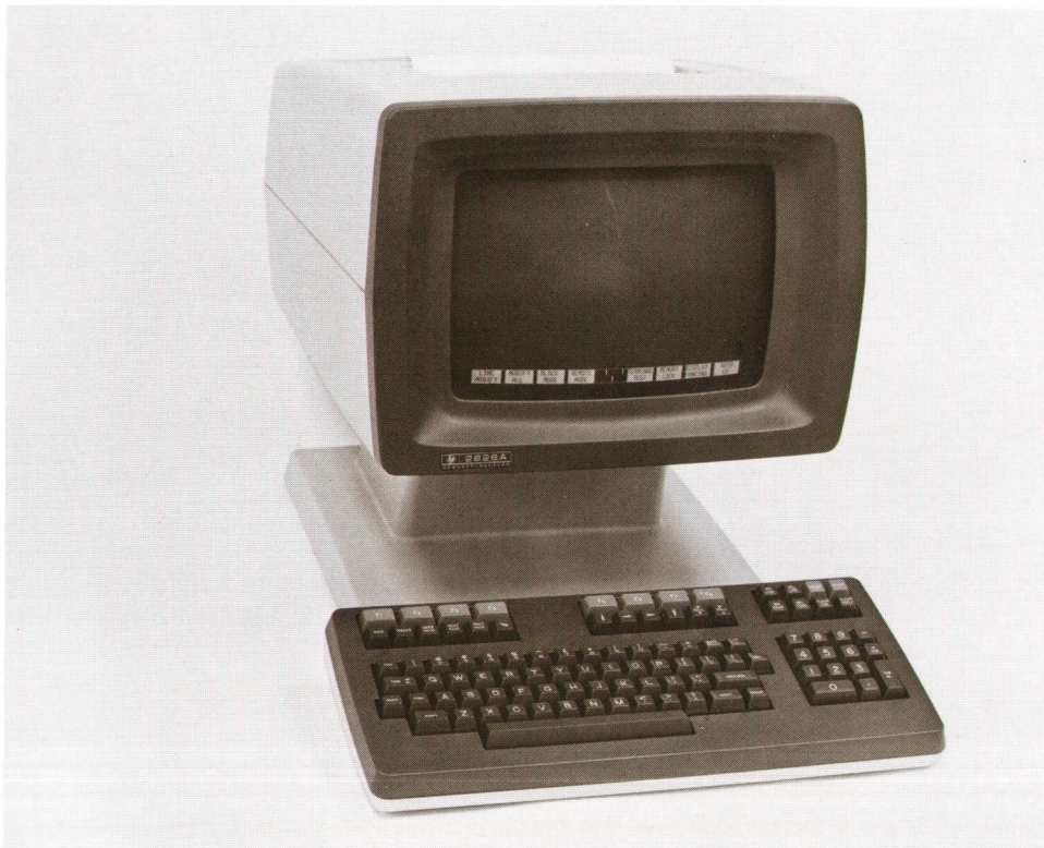
Fig. 1. Model 2626A Display Station is a multi-workspace, multi-window computer terminal that has dual data communications ports. Its capabilities may be configured dynamically as four logically independent virtual terminals. The terminal can handle line lengths up to 160 characters and offers foreign language options and an optional built-in printer.
